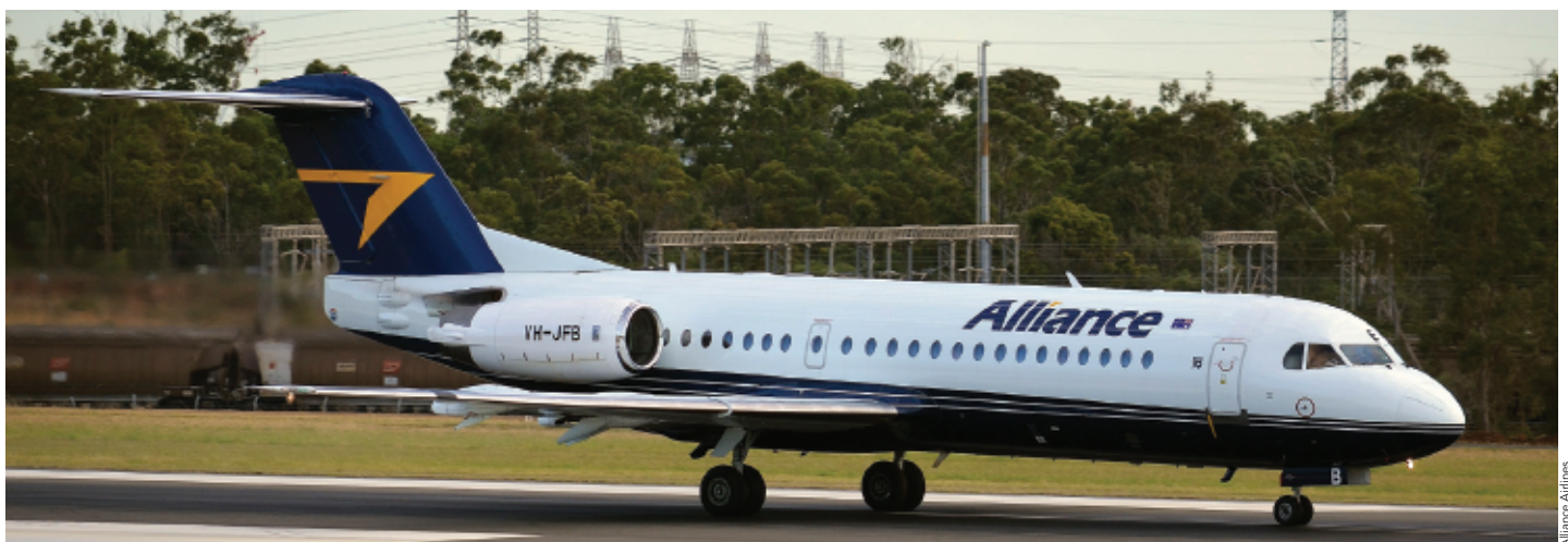
Alliance has upgraded six of its Fokker F70s to the LR variant, so they can make return trips to remote mining sites without refuelling
