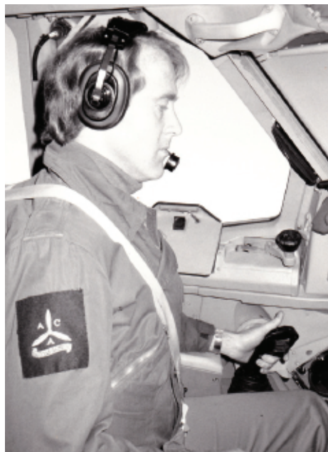
David Learmount gets a feel for the new sidestick on the fly-by-wire A300 testbed
